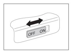
Slide the ON/OFF switch into the "ON" position to activate the radio components.
